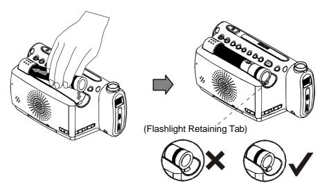
IMPORTANT: The flashlight must be charged in the charging cradle for 24 hours before initial use. When the radio is connected to the AC outlet and the flashlight is properly positioned in the charging cradle the Red "Charging" indicator in the flashlight AUTO /OFF switch comes 'on'.
